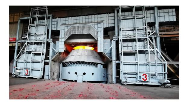
KOBM converter, upgraded from a former BOF converter by Primetals Technologies, started up in the steel plant of HBIS Group Handan Iron and Steel in Handan, China in early November.
